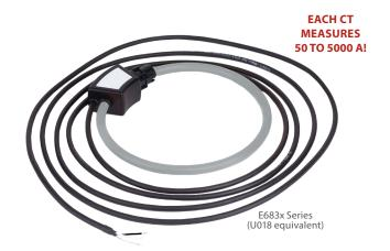
The E683x Series of Rogowski flexible rope style current transducers (CTs) provide secondary AC voltage proportional to the primary (sensed) current. For use with E5xxxA and E2x Series power meters, the E683x Series CTs provide a cost-effective means to transform electrical service amperages to a voltage compatible with monitoring equipment. The flexible core makes it easy to fit in tight enclosures.
