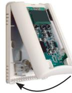
8. Use the switch to select voltage or current output. For CWL model, see Configuration section.
