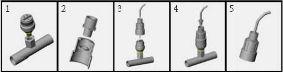
1. Install the remote sensors into the system plumbing (use 3/4" hex to tighten")
