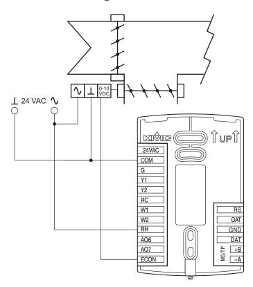
**Connecting power** The AppStat requires an external, 24 volt, AC power source. Use the following guidelines when choosing and wiring transformers.
