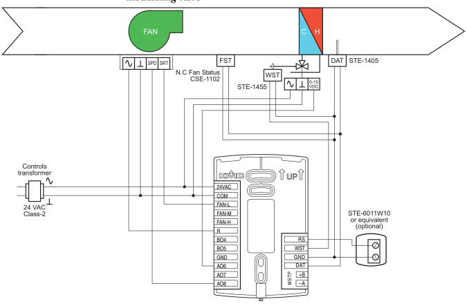
Illustration 6–8 Wiring details: Two-pipe FCU with modulating fan and modulating valve
