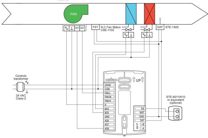
Illustration 6–3 Wiring details: Four-pipe FCU with modulating fan and on/off valves
