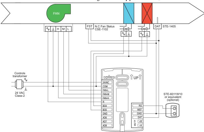
Illustration 6-1 Wiring details: Four-pipe FCU with on/off valves
