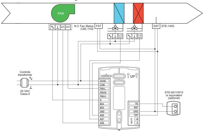
Illustration 6–4 Wiring details: Four-pipe FCU with modulating fan and modulating valves
