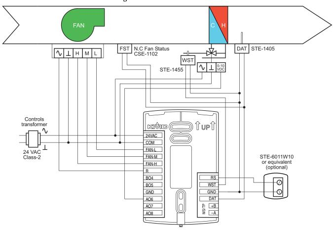
Illustration 6–6 Wiring details: Two-pipe FCU with three-speed fan and modulating valve
