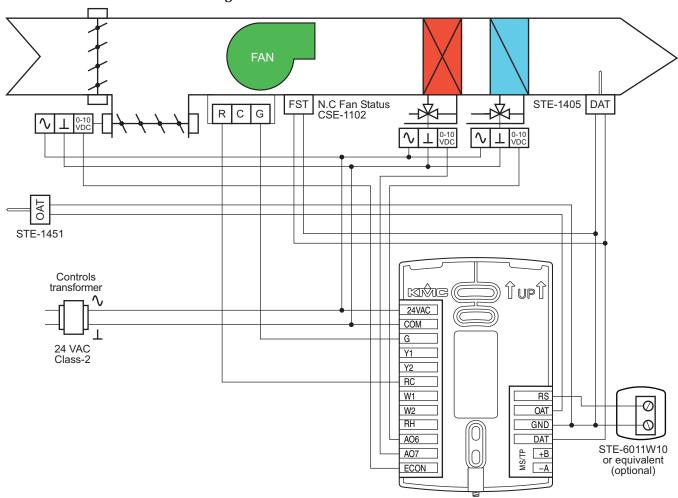
Illustration 6–13 Wiring details: RTU with modulating values for cooling and heating and economizer
