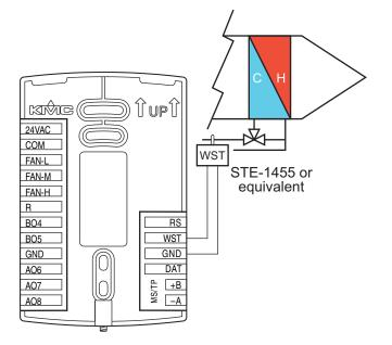
Illustration 2-6 Wiring for a water temperature sensor
