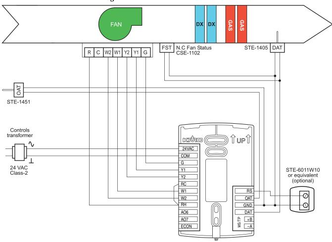
Illustration 6–11 Wiring details: RTU two-stage gas heat and two-stage DX cooling
