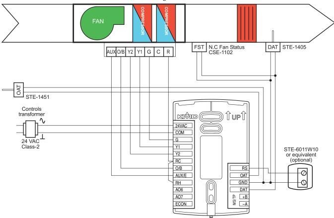
Illustration 6-16 Wiring details: HPU—Three heat, two cool
