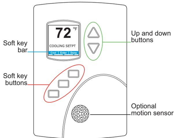
The three buttons below the display are defined by labels in the soft key bar. Typically the buttons are designated for the following functions.
