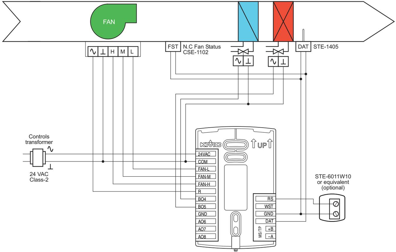
**Fan Coil Unit—Four-pipe with three-speed fan and modulating valves**
