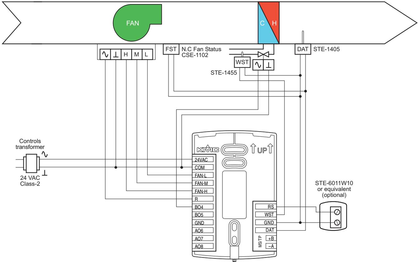
**Fan Coil Unit—Two-pipe with three-speed fan and modulating valve**
