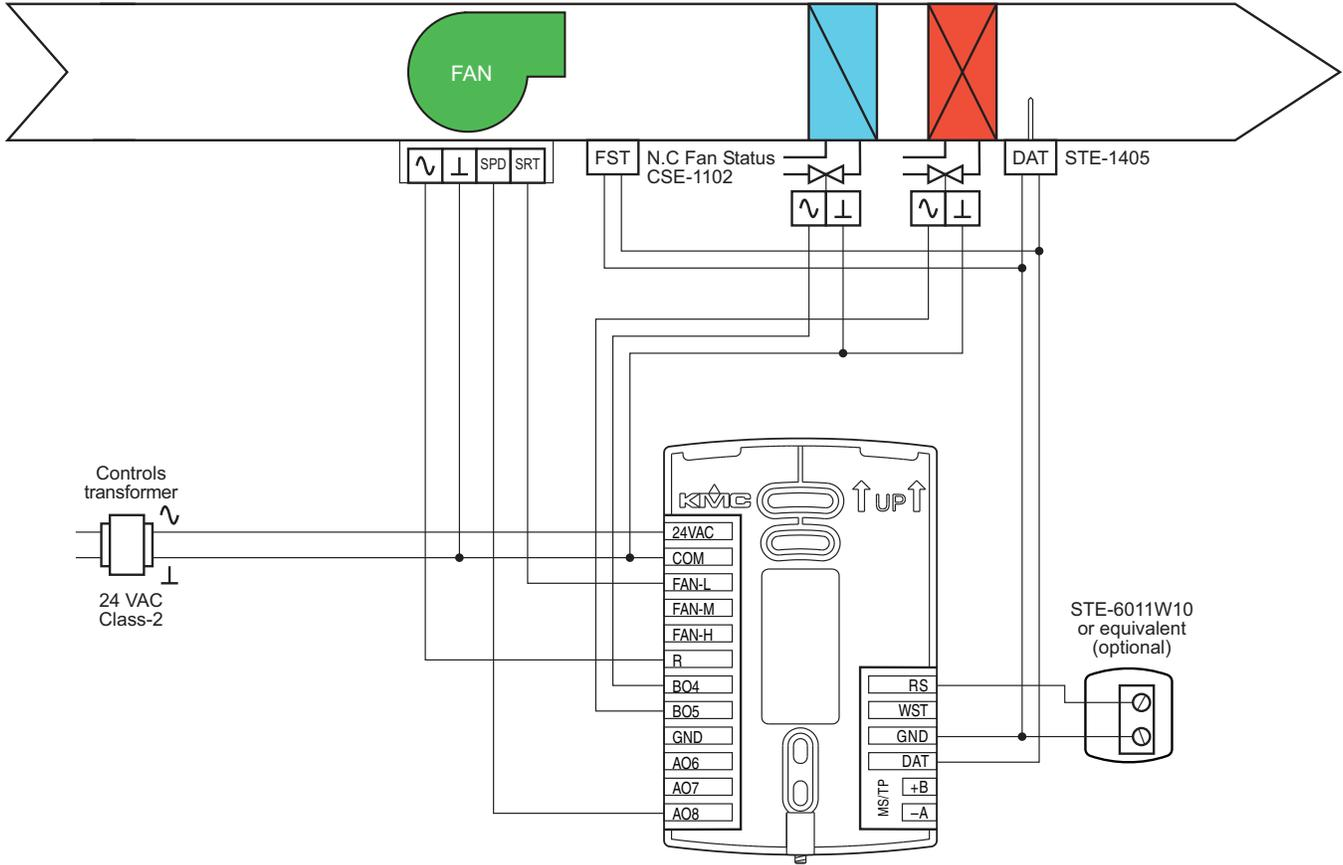
**Fan Coil Unit—Four-pipe with modulating fan and modulating valves**
