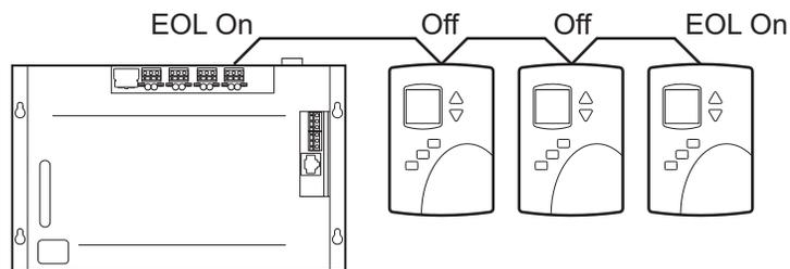
[Location of EOL switch on page 123](#) shows the position of the EOL switches in the AppStat controller.
