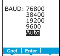
A screenshot of a device display showing Baud rate options. The text "BAUD: 76800" is at the top, followed by "38400", "19200", and "9600". The word "Auto" is highlighted with a black background. At the bottom, there is a blue bar with the text "Cncl" and "Enter" in white, flanked by vertical lines. |
