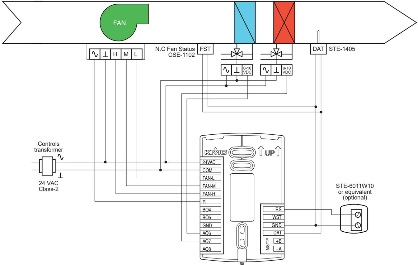
**Fan Coil Unit—Four-pipe with modulating fan and on/off valves**
