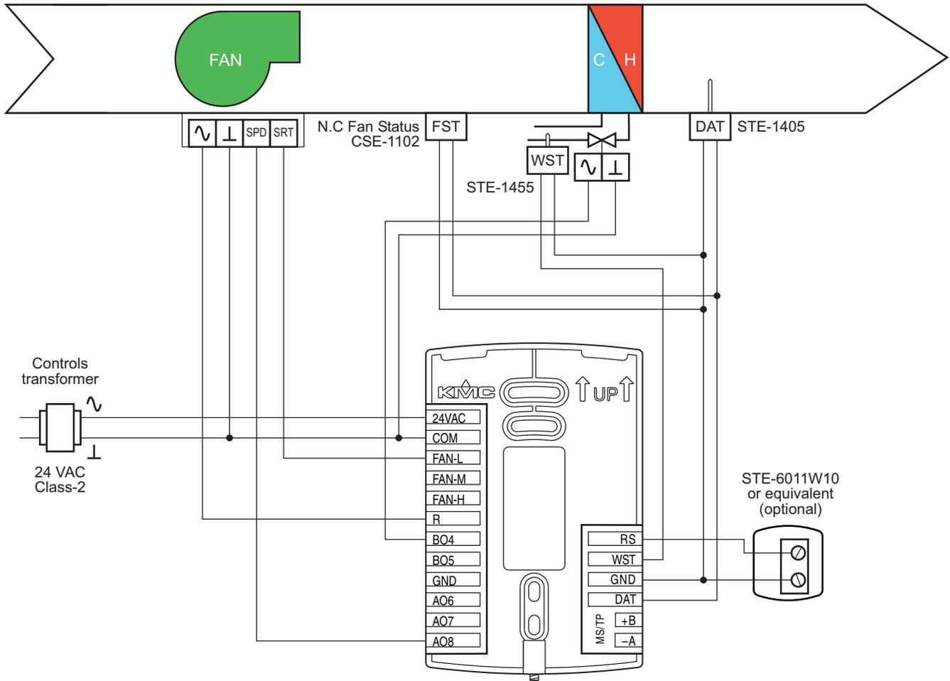
**Fan Coil Unit—Two-pipe with modulating fan and modulating valve**
