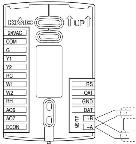
The controllers or devices on the physical ends of the MS/TP wiring segment must have end-of-line (EOL) termination installed for proper network operation. See [Location for end-of-line termination on page 122](#). Set the end-of-line termination to On using the EOL switches.
