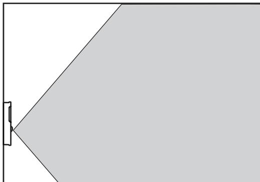
The effective detection range is approximately 10 meters or 33 feet. Factors that may reduce the range include:
