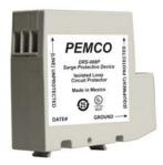
The **PEMCO DRS Series** is a din rail mountable, single pair surge suppression module implementing three-stage hybrid technology. This module addresses overvoltage transients with gas tubes and silicon avalanche components. In addition, sneak currents are mitigated with resettable fuses (PTCs). The PTCs increase resistance several orders of magnitude when overcurrents exceed safe levels. A normal state
