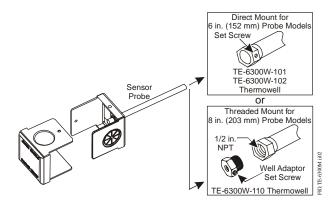
Figure 2: Installing the Well Insertion Sensor
