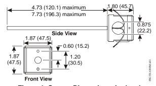
Figure 1: Sensor Dimensions, in. (mm)
