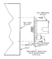
Figure 3: Direct mounting a P32 using the "L" bracket as a mounting flange
