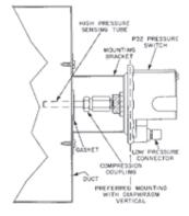
Figure 4: Typical installation for a P32 Switch on duct using Part No. BKT229-1R bracket and direct mounting probe
