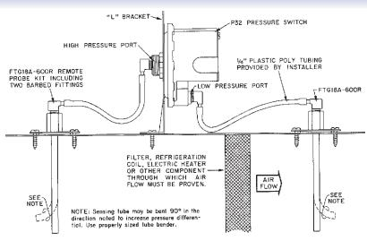
Figure 5: The P32 may be mounted on either a vertical of horizontal surface using an "L" bracket and two FTG18A-600R remote mounted probe kits.
