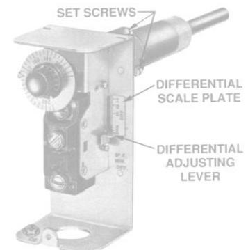
**Fig. 2 -- Illustrated is the A19 with adjustable differential. Note the complete accessibility of the well assembly set screw. After loosening these screws, the control can be quickly removed from the well.**
