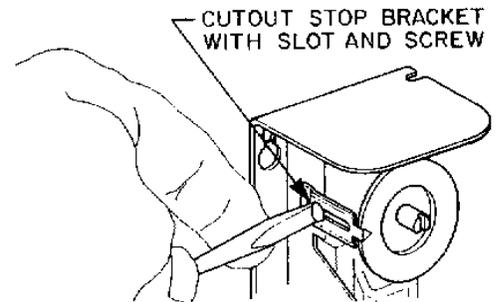
**Fig. 5 — The controls have a screw type cutout stop. The stop screw must be loosened and moved to the stop setting desired. Tighten screw after setting is made.**
