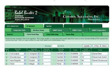
Configuration of the gateway is done via the web pages served by the internal web server. The user simply fills in templates. The entire configuration is saved in the internal Flash file system in XML format. This file may be exported to replicate additional copies of the configured device, or for backup.
