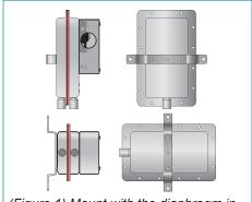
(Figure 1) Mount with the diaphragm in any vertical plane to obtain the lowest specified operating set point.
