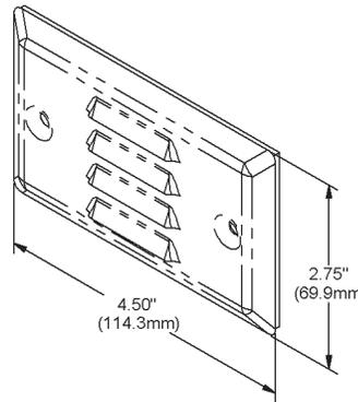
**Fig 3:** Horizontal Louvered Temperature Sensor
