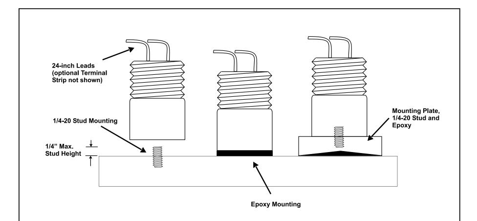
Model 140 Vibration Transmitter Mounting Guidelines
