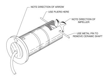
Figure 2: Impeller Assembly and Shaft
