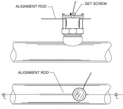
Figure 2: Alignment of Flow Sensor 220BR and 220SS
