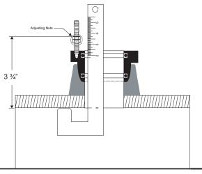
Figure 1: Installation for 220BR and 220SS
