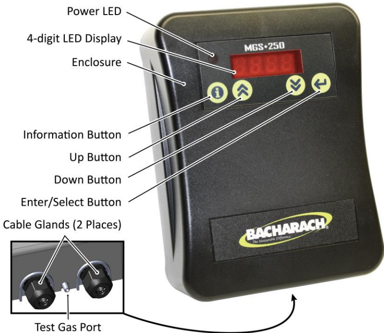
Figure 1. MGS-250 Components
