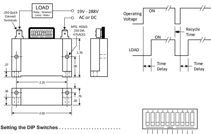
The DIP switches are used to set the time delay period between 1 and 1024 seconds. The timer has an internal 1 second delay, opening of the DIP switches adds their corresponding value to that internal delay. The switches to the right are all opened for a total delay of 1023 seconds, adding that to the internal 1 second provides the full 1024 seconds. Any time delay from 1 to 1024 seconds can be achieved by opening the appropriate switches.
