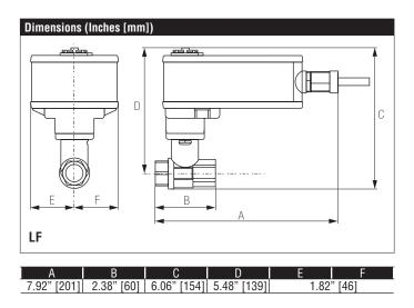
Modulating, Non-Spring Return, 24 V, for 2 to 10 VDC or 4 to 20 mA
