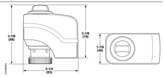
Figure 7. Dimensions of the SSB Actuator in Inches (Millimeters).
