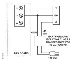
Figure 5. Terminal Connections of the SSB61U.
