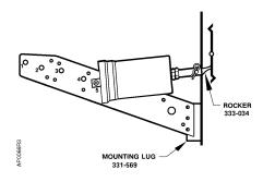
Figure 14. Frame Mounting Normally Closed Damper.
