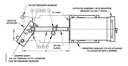
Figure 8. Fixed Mounted Actuator Assembly. Dimensions in Inches (Millimeters).
