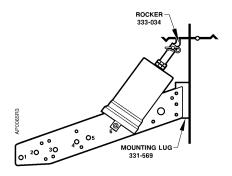
Figure 13. Frame Mounting Normally Open Damper.
