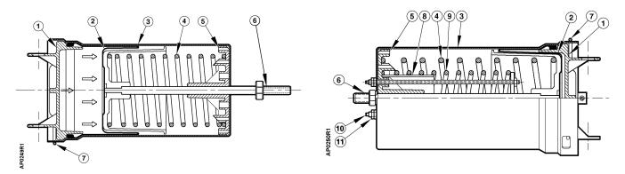
Figure 3. Standard Actuator.
