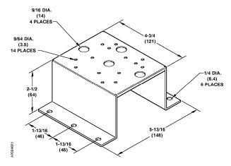
Figure 9. Offset Mounting Bracket 333-176. Dimensions in Inches (Millimeters).
