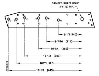
Figure 5. Actuator Mounting Plate 331-623. Dimensions in Inches (Millimeters).
