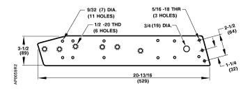
Figure 12. Actuator Mounting Plate 331-623, 1/4-Inch (6 mm) Thick.
