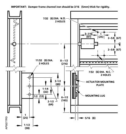
Figure 10. Frame Mounting Dimensions. Dimensions in Inches (Millimeters).
