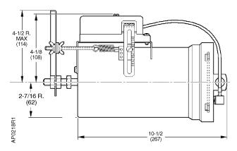
Figure 15. Dimensions with the RL 147 Positioning Relay Mounted.
