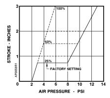
Figure 2. Hesitation Actuator Adjustment.
