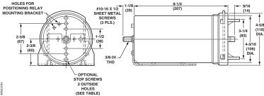
Figure 16. Bracket Mounted Actuator 331-2911 (Typical). Dimensions in Inches (Millimeters).
