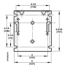
Figure 11. Mounting Bracket Dimensions. Dimensions in Inches (Millimeters).
