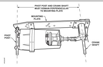
Figure 7. Perpendicular Mounting.
