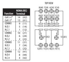
\*Observe polarity for relays with DC coil voltages only
