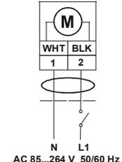
Important - Do not install multiple VAS-27 Series actuators connected to the same mechanical load. Master-Slave application of DS-27 Series Actuators requires that each actuator be connected to independent loads.
