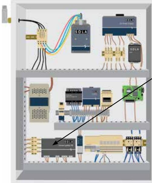
*The SDU AC - A Series provides back-up protection for sensitive equipment in a control panel.*
