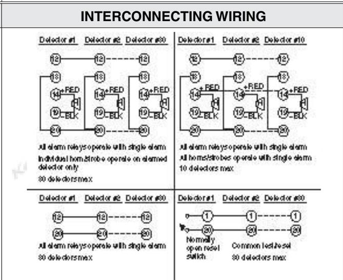
**CAUTION:** For terminals (7, 8, 18), (6, 16, 17), and (13, 14) do not use looped wire under terminals. Break wire run to provide supervision of connections.
