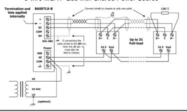
For MS/TP devices that use a power source separate from the BASRTLX-B
