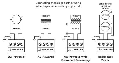
**WARNING:** Internally, this device utilizes a half-wave rectifier and therefore can only share the same AC power source with other half-wave rectified devices. Sharing a common DC power source is also possible. Sharing AC power with full-wave rectified devices is NOT recommended. Devices powered from a common AC source could be damaged if a mix of half-wave and full-wave rectified devices exists.
