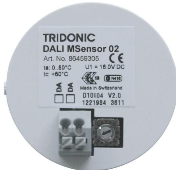
Figure 159: Set MSensor group dial to position 'F'.
