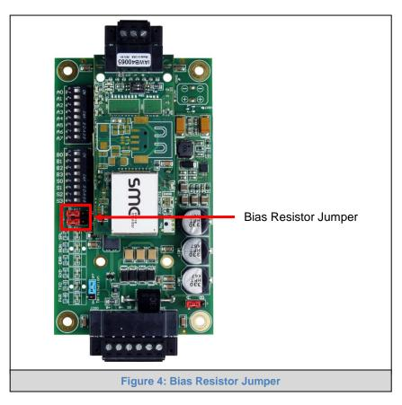
The FieldServer bias resistors are used to keep the RS-485 bus to a known state, when there is no transmission on the line (bus is idling), to help prevent false bits of data from being detected. The bias resistors typically pull one line high and the other low - far away from the decision point of the logic.
