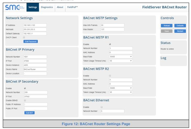
NOTE: The FieldPoP™ tab FieldPoP™ (see Figure 12) allows users to connect to the SMC Cloud, Sierra Monitor's device cloud solution for IIoT. The SMC Cloud enables secure remote connection to field devices through a FieldServer and its local applications for configuration, management, maintenance. For more information about the SMC Cloud, refer to the SMC Cloud Start-up Guide.
