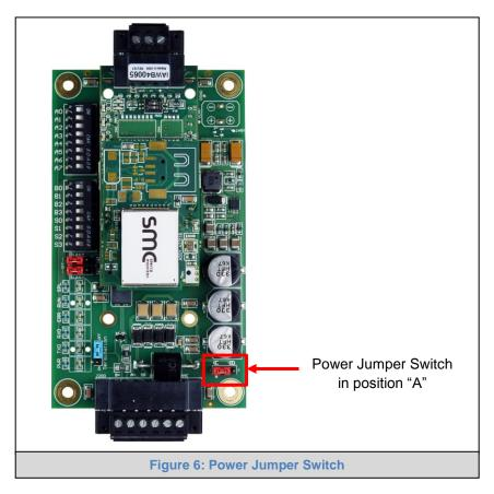
The FieldServer Carrier Board power jumper is set to position A by default but can be changed to position B for other power supply requirements.
