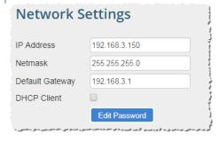
The IP settings for the router are also used by both BACnet/IP connections. The IP settings can be changed in the Network Settings section as shown.
