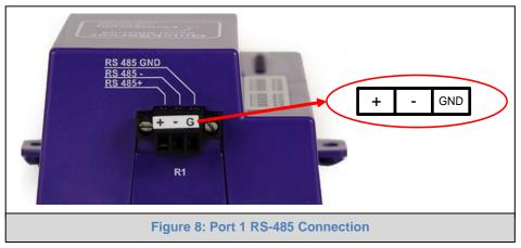
The following Baud Rates are supported on the R1 Port: 9600, 19200, 38400, 57600, 76800, 115200
