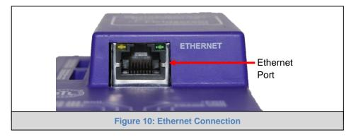
The Ethernet Port is used both for BACnet Ethernet and BACnet/IP communications. It is also used for configuring the router from a Web page.
