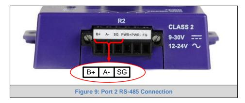
Connect to the 3 pins on the left-hand-side of the 6 pin connector as shown.
