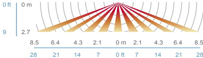
**Note:** Sensor's screw axis is offset 7.5° from a long detection segment
